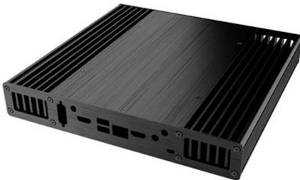
This enclosure enables a fully fanless working PC with Intel NUC7i5DNBE / NUC7i3DNBE / NUC7i5DNKE / NUC7i3DNKE / NUC7i3DNHE NUC mainboard. Perfect for HTPC, Digital Signage or Server applications.
